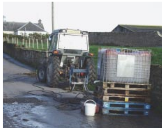
Figure 1: Temporary cleansing and disinfection point at farm entrance during FMD 2001. The tractor powers the pressure washer. (Picture courtesy David Logue)
