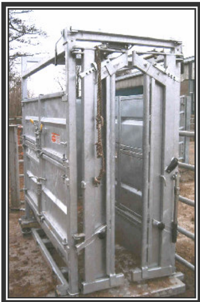
Figure 5.21.: A self-catching head yoke with parallel stanchions used primarily for cattle of calm temperament.
