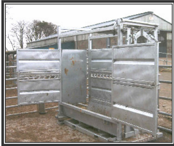
Figures 5.25. and 5.26.: A crush that provides unobstructed access to the animal with no supports against which a handler may be trapped.
