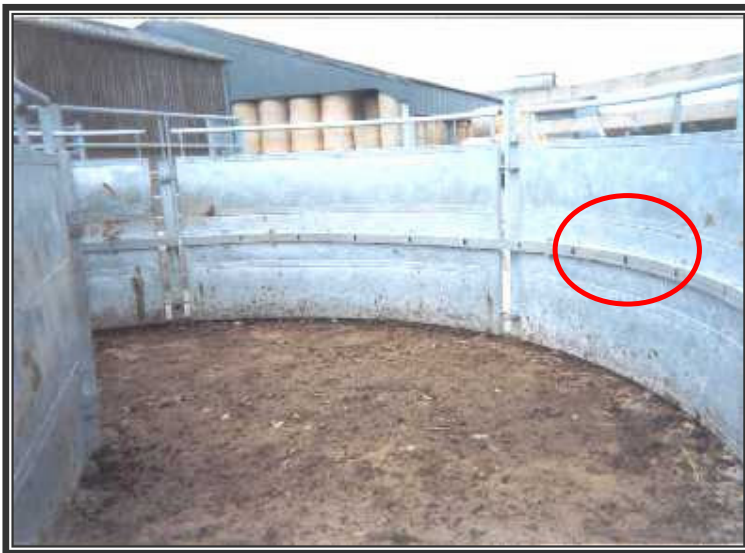
Figure 5.7.: Outer wall of a curved forcing pen with holes for a spring loaded pin to prevent accidental movement of the forcing gate.
